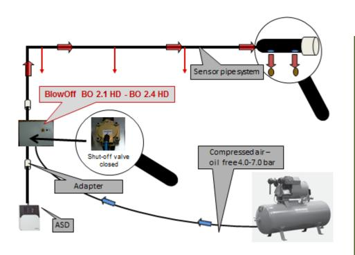
Figure : Air-blast process with BlowOff
